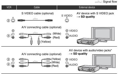
\* When connecting the VCR to a monaural device, connect the yellow plug of the A/V connecting cable to the video jack on the device, and connect the white (left channel) or red (right channel) plug to the audio jack on the device.
